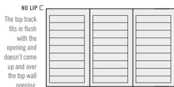
**NO LIP** The top track fits in flush with the opening and doesn't come up and over the top wall opening.
